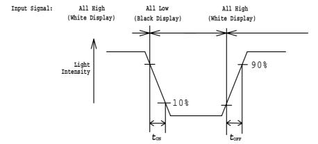
$t_{\mathrm{ON}}$ : Turn on time is the time for a photo detector output waveform to go from 90% value to 10% of its maximum.
